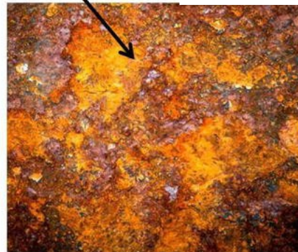
Surface damage due to corrosion and oxidation
